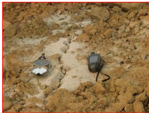
Fig.30. Liquefaction feature by the Tarlay earthquake
